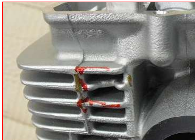
Figure 3: Cylinder Head with Misrun Defect
